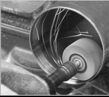
Deburring a tube end with a stem-mounted flap wheel. For those situations where a die grinder is the most appropriate tool for the job, flap wheels offer effective solutions for a wide variety of cleaning, deburring, blending, and finishing applications.
