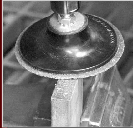
Removing saw marks from a cut end of stainless bar with a blending disc. When more aggression is required for removing deeper tool marks or surface imperfections, blending discs offer a solution.
