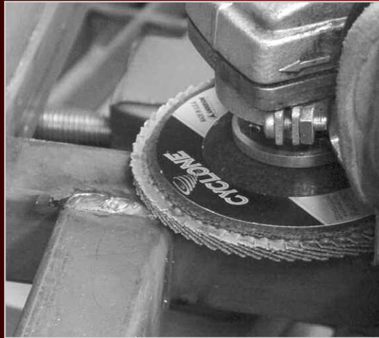
Removing heat discoloration from a stainless sheet with an Anderlex surface prep disc. These are effective tools for removing oxides, residue, and discoloration from sheet metal after welding.
