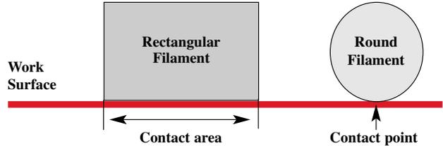
Rectangular filaments are stiffer and provide a greater contact area with the work surface. These filaments should be used in high aggression applications where less conformability is required.
