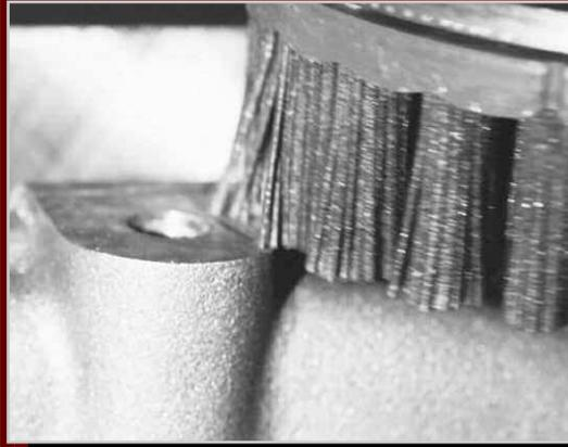
Disc brushes are ideal for deburring flat surfaces after face milling. On such parts, all burred edges are on the same plane and are easily deburred.
