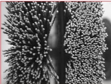
Proper selection of brush density and trim length is a critical element in optimizing the output of a brushing operation. While high density/short trim brushes offer better cycle times and longer brush life, they are not effective in operations requiring a high degree of brush conformability. The following illustration highlights the differences between 10" x 2" arbor hole wheel brushes versus the 10" x 5-1/4" arbor hole version.
