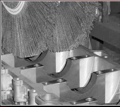
Large diameter wheel brushes are used to focus significant deburring energy on targeted edges. The steel inserts in this aluminum engine component have a severe burr condition requiring the aggression of wheel brushes.
