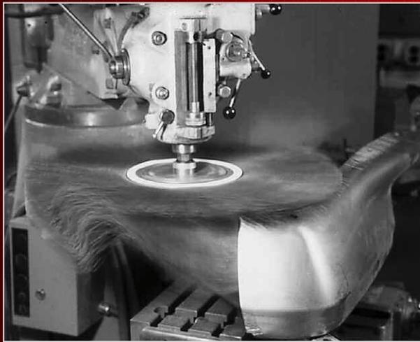
CNC equipment allows disc brushes to be used for in-machine deburring. In such situations, secondary deburring operations can be completely eliminated.
